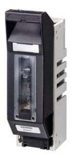
LV HRC FUSE BASE AC 690V, WITH SLEWING EQUIPMENT SIZE 00 160A 1POLE WITH SREW-TYPE TERMINAL CONNECTION WITH CLAW ATTACHMENT
