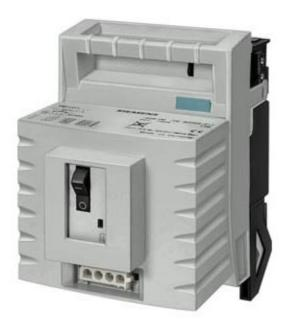
FUSE-SWITCH-DISCONNECTOR SIZE 2, I = 400 A, U = 690 V, FOR SURFACE MOUNT. AND INST., WITH FUSE MONITORING, FLAT PAD CONNECTION M10, FUSE SIZE NH2, HANDLE UNIT GRAY
