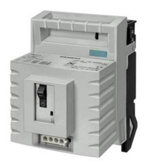
FUSE-SWITCH-DISCONNECTOR I = 630 A, U = 690 V, FOR 60MM BUSBAR SYSTEMS WITH FUSE MONITORING, FLAT PAD CONNEC. M12, OPTIONAL BOTTOM OR TOP, FUSE SIZE NH3
