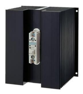
SEMI-COND. CONTACTOR 3RF2,1-PH. AC51 90A 40 DEGREE C 48-600 V / 4-30 V DC RING CABLE CONNECTION BLOCKING VOLTAGE 1200 V
