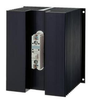
SEMI-COND. CONTACTOR 3RF2,1-PH. AC 51 90A / AC15 30A 40 DEG. C 48-600 V / 110-230 V AC INSTANTANEOUS SWITCHING
