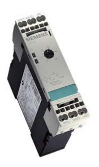
MULTIFUNCTION TIME RELAY IN CAGE-CLAMP TECH. 1 NO CONTACT DELAYED, 1 NO CONTACT NON-DELAYED, 3S...60S, AC/DC 24V, AC 200...240V
