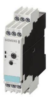
TEMPERATURE MONITORING RELAY FOR PT100, EXCEEDING OF 1 THRESH. VAL., WIDTH 22ND5 MM 0 C - 200 C, 24V AC/DC 1 NO + 1 NC, CLOSED-CIRC.PRINC. CAGE-CLAMP - CONNECTION
