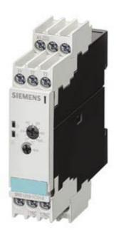
TEMPERATURE MONITORING RELAY FOR PT100, EXCEEDING OF 1 THRESH. VAL., WIDTH 22ND5 MM 0 C-200 C, 110-120/220-240V AC 1 NO + 1 NC, CLOSED-CIRC.PRINC. CAGE-CLAMP - CONNECTION
