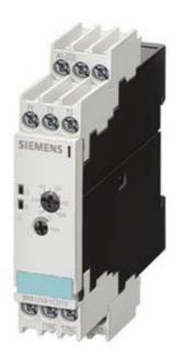
TEMPERATURE MONITORING RELAY PT1000 OVERRANGE 1 THRESHOLD, WIDTH 22.5 MM 0 DEG. C TO 200 DEG. C 24 V AC/DC, 1NO+1NC, CLOSED-CIRCUIT SYSTEM CAGE CLAMP TERMINAL
