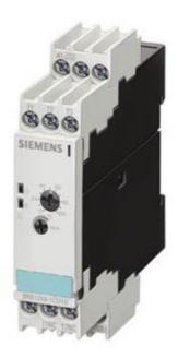
TEMPERATURE MONITORING RELAY FOR PT100, UNDERSHOOTING OF 1 THRESH. VAL., WIDTH 22ND5 MM 0 C-100 C, 110-120/220-240V AC 1 NO + 1 NC, CLOSED-CIRC.PRINC. SCREW CONNECTION
