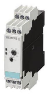
TEMPERATURE MONITORING RELAY FOR PT100, UNDERSHOOTING OF 1 THRESH. VAL., WIDTH 22ND5 MM 0 C-200 C, 110-120/220-240V AC 1 NO + 1 NC, CLOSED-CIRC.PRINC. SCREW CONNECTION
