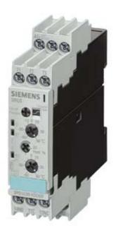
TEMPERATURE MONITORING RELAY FOR PT100, EXCEEDING OF 2 THRESH. VAL., WIDTH 22ND5 MM 0 C - 200 C, 24V AC/DC 1 NO+1 W, LOAD + CL.-CIRC.CURR. SCREW CONNECTION
