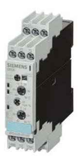
TEMPERATURE MONITORING RELAY FOR PT100, EXCEEDING OF 2 THRESH. VAL., WIDTH 22ND5 MM -50 C-50 C, 110-120/220-240V AC 1 NO+1 W, LOAD + CL.-CIRC.CURR. SCREW CONNECTION
