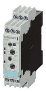
TEMPERATURE MONITORING RELAY FOR PT100, EXCEEDING OF 2 THRESH. VAL., WIDTH 22ND5 MM 0 C-200 C, 110-120/220-240V AC 1 NO+1 W, LOAD + CL.-CIRC.CURR. CAGE-CLAMP - CONNECTION
