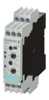
TEMPERATURE MONITORING RELAY FOR PT100, UNDERSHOOTING OF 2 THRESH. VAL., WIDTH 22ND5 MM 0 C-200 C, 110-120/220-240V AC 1 NO+1 W, LOAD + CL.-CIRC.CURR. SCREW CONNECTION
