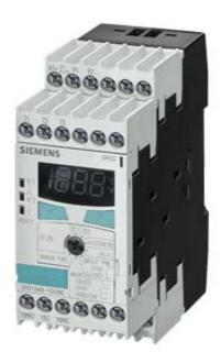
TEMPERATURE MONITORING RELAY PT100/1000 KTY83/84, NTC 2 THRESH. VAL., DIGITAL -50 C - 500 C, 24V AC/DC 2 X 1 W + 1 NO, WIDTH 45 MM SCREW CONNECTION
