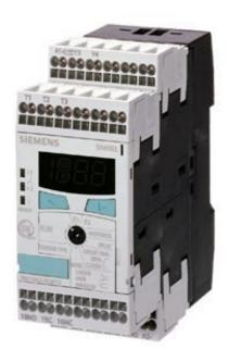
TEMPERATURE MONITORING RELAY PT100/1000 KTY83/84, NTC 2 THRESH. VAL., DIGITAL -50 C - 500 C, 24-240V AC/DC 2 X 1 W + 1 NO, WIDTH 45 MM CAGE-CLAMP - CONNECTION
