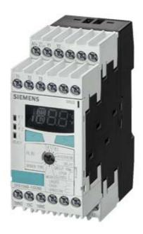
TEMPERATURE MONITORING RELAY PT100/1000 KTY83/84, NTC, 2 THRESHOLDS, DIGITAL, -50 DEGREES C TO 750 DEGREES C (SENSOR-DEPENDENT), 24 V AC/DC, 2 X 1 CO + 1 NO, WIDTH 45 MM, SCREW TERMINAL
