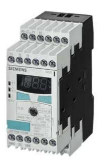
TEMPERATURE MONITORING RELAY PT100/1000 KTY83/84, NTC, 2 THRESHOLDS, DIGITAL, -50 DEGREES C TO 750 DEGREES C (SENSOR-DEPENDENT), 24 V TO 240 V AC/DC, 2 X 1 CO + 1 NO, WIDTH 45 MM, SCREW TERMINAL
