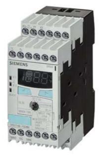
TEMPERATURE MONITORING RELAY THERMOCOUPLE J,K,T,E,N,S,R,B, 2 THRESHOLDS, DIGITAL, -99 DEGREES C TO 1800 DEGREES C (SENSOR-DEPENDENT), 24 V AC/DC, 2 X 1 CO + 1 NO,
