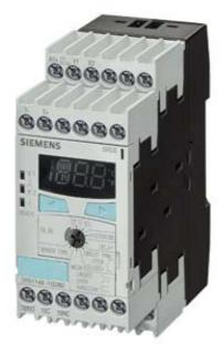
TEMPERATURE MONITORING RELAY THERMOCOUPLE J,K,T,E,N,S,R,B, 2 THRESHOLDS, DIGITAL, -99 DEGREES C TO 1800 DEGREES C (SENSOR-DEPENDENT), 24 V TO 240 V AC/DC, 2 X 1 CO + 1 NO, WIDTH 45 MM,
