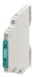
INTERFACE CONVERTER AC/DC 24 V, 2 WAY SEPARATION ON: 0 TO 10 V OFF: 4 TO 20 MA SCREW CONNECTION
