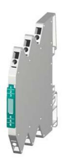
INTERFACE CONVERTER AC/DC 24 V, 3 WAY SEPARATION ON: 4 TO 20 MA OFF: 4 TO 20 MA SCREW CONNECTION
