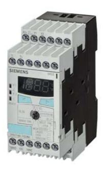
TEMPERATURE MONITORING RELAY PT100/1000, KTY83/84, NTC 2 THRESHOLD VALUES, DIGITAL -58 DEGR.F TO 932 DEGR.F 24-240V AC/DC
