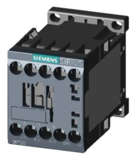
CONTACTOR, AC-3, 4KW/400V, 1NC, DC 24V, 3-POLE, SZ S00 SCREW TERMINAL MULTI-UNIT PACKAGING PACKAGE = 40 UNITS
