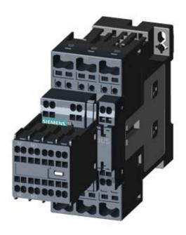
CONTACTOR, AC-3, 5.5KW/400V, 2NO+2NC, DC 24V, 3-POLE, SZ S0 SPRING-LOADED TERMINAL REMOVABLE AUX. SWITCH PACKAGE = 40 UNIT(S)
