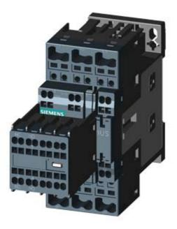
CONTACTOR, AC-3, 11KW/400V, 2NO+2NC, AC 230V 50HZ, 3-POLE, SZ S0 SPRING-LOADED TERMINAL REMOVABLE AUX. SWITCH PACKAGE = 40 UNIT(S)
