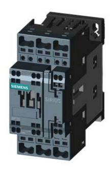
CONTACTOR, AC-3, 15KW/400V, 1NO+1NC, AC 230V 50HZ, 3-POLE, SZ SO SPRING-LOADED TERMINAL
