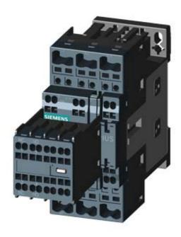
CONTACTOR, AC-3, 15KW/400V, 2NO+2NC, AC 230V 50HZ, 3-POLE, SZ S0 SPRING-LOADED TERMINAL REMOVABLE AUX. SWITCH PACKAGE = 40 UNIT(S)
