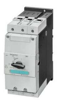
CIRCUIT-BREAKER SIZE S3 A-RELEASE 36...50 A, N-RELEASE 650 A MOTOR PROTECTION, CLASS 10 SCREW CONNECTION STANDARD BREAKING CAPACITY REUSABLE PACKING PACKING = 15 ITEMS
