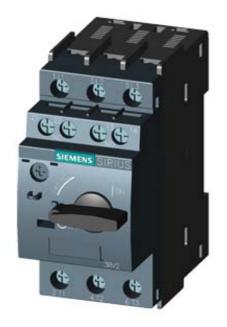
CIRCUIT-BREAKER SZ S00, FOR MOTOR PROTECTION, CLASS 10, A-REL. 0.14...0.2A,N-REL.2.6A, SCREW CONNECTION, STANDARD SW. CAPACITY, W. TRANSVERSE AUX. SWITCH 1NO+1NC MULTI-UNIT PACKAGING PACKAGE = 12 UNITS
