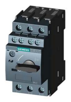
CIRCUIT-BREAKER SZ S00, FOR MOTOR PROTECTION, CLASS 10, A-REL. 0.14...0.2A,N-REL.2.6A, SCREW CONNECTION, STANDARD SW. CAPACITY, W. TRANSVERSE AUX. SWITCH 1NO+1NC
