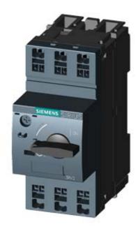
CIRCUIT-BREAKER SZ S00, FOR MOTOR PROTECTION, CLASS 10, A-REL.0.18...0.25A,N-REL.3.3A SPRING-L. CONNECTION STANDARD SWITCHING CAPACITY REUSABLE PACKING, PACKAGE = 34 UNITS
