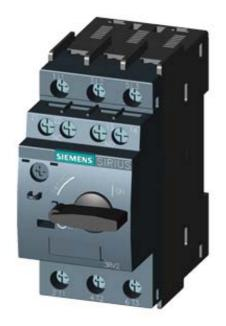
CIRCUIT-BREAKER SZ S00, FOR MOTOR PROTECTION, CLASS 10, A-REL. 0.22...0.32A, N-RELEASE4.2A SCREW CONNECTION, STANDARD SW. CAPACITY, W. TRANSVERSE AUX. SWITCH 1NO+1NC MULTI UNIT PACKAGING PACKAGE = 12 UNITS
