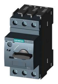
CIRCUIT-BREAKER SZ S00, FOR MOTOR PROTECTION, CLASS 10, A-REL. 0.7...1A, N-REL. 13A, SCREW CONNECTION, STANDARD SWITCHING CAPACITY REUSABLE PACKING, PACKAGE = 43 UNITS
