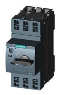
CIRCUIT-BREAKER SZ S00, FOR MOTOR PROTECTION, CLASS 10, A-REL.0.9...1.25A, N-REL.16A, SPRING-L. CONNECTION STANDARD SWITCHING CAPACITY MULTI UNIT PACKAGING PACKAGE = 8 UNITS
