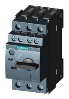
CIRCUIT-BREAKER SZ S00, FOR MOTOR PROTECTION, CLASS 10, A-REL.1.1...1.6A, N-RELEASE 21A, SCREW CONNECTION, STANDARD SW. CAPACITY, W. TRANSVERSE AUX. SWITCH 1NO+1NC REUSABLE PACKAGING PACK = 43 UNITS
