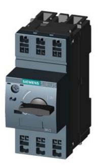
CIRCUIT-BREAKER SZ S00, FOR MOTOR PROTECTION, CLASS 10, A-REL. 1.4...2A, N-RELEASE 26A, SPRING-L. CONNECTION STANDARD SW. CAPACITY MULTI-UNIT PACKAGING PACKAGE = 8 UNITS
