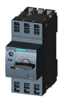
CIRCUIT-BREAKER SZ S00, FOR MOTOR PROTECTION, CLASS 10, A-REL. 1.4...2A, N-RELEASE 26A, SPRING-L. CONNECTION STANDARD SW. CAPACITY
