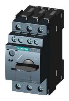
CIRCUIT-BREAKER SZ S00, FOR MOTOR PROTECTION, CLASS 10, A-REL. 1.8...2.5A, N-RELEASE 33A SCREW CONNECTION, STANDARD SW. CAPACITY, W. TRANSVERSE AUX. SWITCH 1NO+1NC MULTI-UNIT PACKAGE = 12 UNITS
