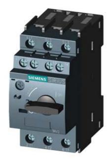
CIRCUIT-BREAKER SZ S00, FOR MOTOR PROTECTION, CLASS 10, A-REL. 2.2...3.2A, N-AUSL.42A SCREW CONNECTION, STANDARD SW. CAPACITY W. TRANSVERSE AUX. SWITCH 1NO+1NC MULTI-UNIT-PACKAGING PACKAGE= 24 PCS
