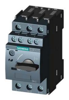
CIRCUIT-BREAKER SZ S00, FOR MOTOR PROTECTION, CLASS 10, A-RELEASE 2.8...4A, N-RELEASE 52A, SCREW CONNECTION, STANDARD SW. CAPACITY, W. TRANSVERSE AUX. SWITCH 1NO+1NC MULTI-UNIT PACKAGE = 12 UNITS
