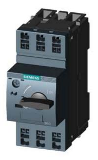
CIRCUIT-BREAKER SZ S00, FOR MOTOR PROTECTION, CLASS 10, A-REL. 2.8...4A, N-REL. 52A, SPRING-L. CONNECTION, STANDARD SWITCHING CAPACITY REUSABLE PACKING, PACKAGE = 34 UNITS
