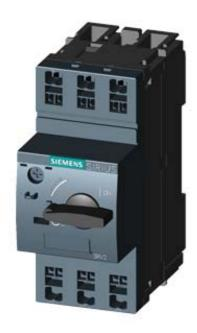
CIRCUIT-BREAKER SZ S00, FOR MOTOR PROTECTION, CLASS 10, A-RELEASE 5.5...8A, N-RELEASE 104A, SPRING-L. CONNECTION, STANDARD SW. CAPACITY
