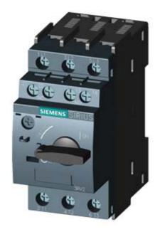
CIRCUIT-BREAKER SZ S00, FOR MOTOR PROTECTION, CLASS 10, A-RELEASE 7...10A, N-RELEASE 130A, SCREW CONNECTION, STANDARD SW. CAPACITY W. TRANSVERSE AUX. SWITCH 1NO+1NC MULTI-UNIT PACKAGE = 12 UNITS
