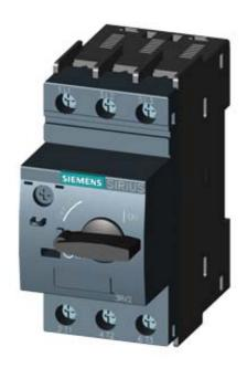
CIRCUIT-BREAKER SZ S0, FOR MOTOR PROTECTION, CLASS 10, A-RELEASE 27...32A, N-RELEASE 400A, SCREW CONNECTION, STANDARD SW. CAPACITY,
