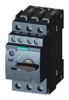
CIRCUIT-BREAKER SZ S0, FOR MOTOR PROTECTION, CLASS 10, A-RELEASE 27...32A, N-RELEASE 400A, SCREW CONNECTION, STANDARD SW. CAPACITY, W. TRANSVERSE AUX. SWITCH 1NO+1NC
