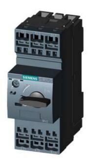
CIRCUIT-BREAKER SZ S0, FOR MOTOR PROTECTION, CLASS 10, A-RELEASE 23...28A, N-RELEASE 364A, SPRING-L. CONNECTION, STANDARD SW. CAPACITY,
