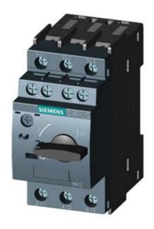
CIRCUIT-BREAKER SZ S0, FOR MOTOR PROTECTION, CLASS 10, A-RELEASE 30...36A, N-RELEASE 432A, SCREW CONNECTION, STANDARD SW. CAPACITY, W. TRANSVERSE AUX. SWITCH 1NO+1NC
