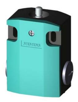
BASIC SWITCH FOR POSITION SWITCH 3SE51, ATEX METAL ENCLOSURE 56MM WIDE DEVICE CONNECTION 3X (M20X1.5) 1NO/ 2NC SNAP-ACTION CONTACTS W/O ACTUATOR HEAD
